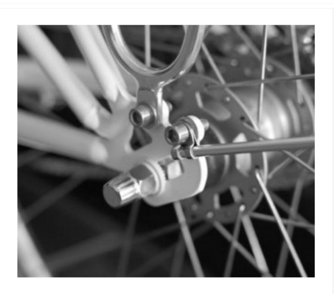
Attaching the fender at the seatstay bridge with a bracket:
